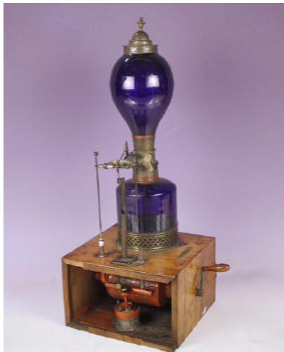
Fig. 7: A hydrogen lighter with a cylinder electrostatic machine and a Lyden jar. (Private collection).
